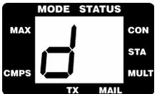
'd' doesn't stand for an actual mode, but will light during special telemetry and data conversion applications.
