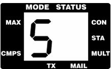
'S' will light when you're using Signal Identification and Acquisition mode (SIAM™) to identify signals.
