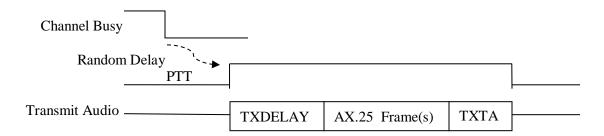
Transmit timing is determined by 4 parameters with these traditional names and typical default values.
